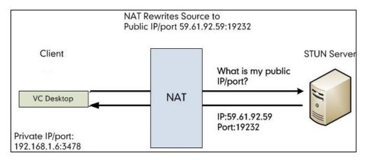
Capturing packets after you enable the STUN feature, you can find that the Yealink VC Desktop sends Binding Request to the STUN server, and then mapped IP address and port is placed in the Binding Response: Binding Success Response MAPPED-ADDRESS: 59.61.92.59:19232.
