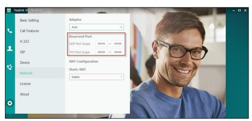
3. Configure the TCP port range in the TCP Port Scope field.
