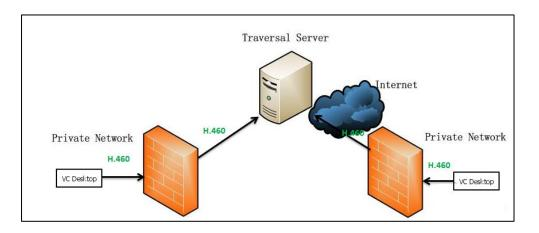
The following illustration shows how a H.460 traversal server works between two enterprise locations.
